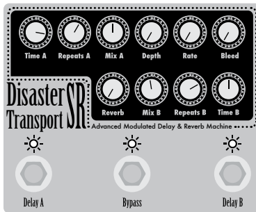
Parallel with no modulation or reverb
