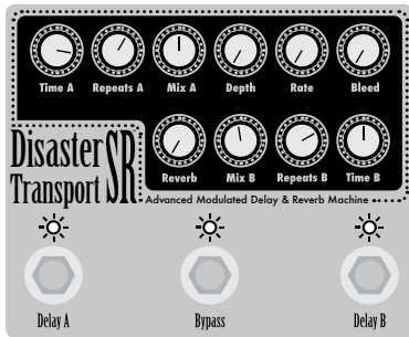
Parallel with no modulation or reverb
